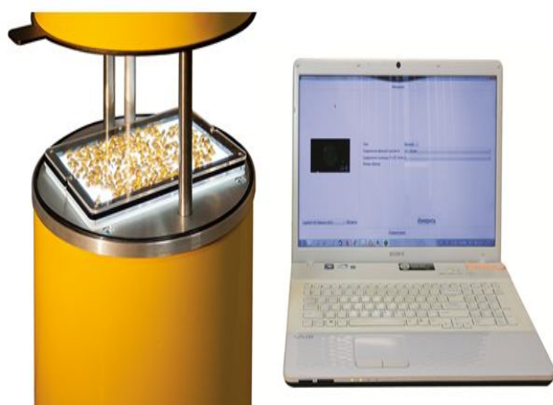
Fig. 2. Diaphanoscope "Yantar" with a cartridge and a computer
